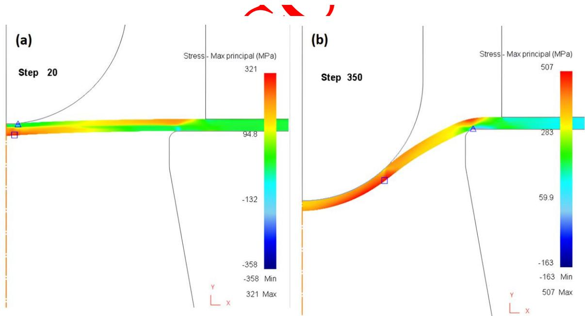
**Figure 16.** Principal stresses generated during the Erichsen test simulations: a) punch advancement = 0.4 mm, b) punch advancement = 7.0 mm
