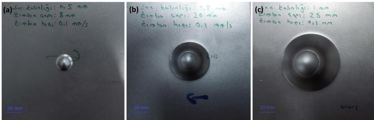
**Figure 21.** Deformations occurring after the Erichsen cupping tests on the DC04 steel sheet samples; a) the  $P_D = 8$  mm, b) the  $P_D = 20$  mm, c) the  $P_D = 25$  mm
