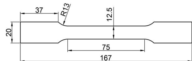
**Figure 1.** Dimensions of the tensile test sample (in mm) as per ISO 6892-1:2009 standards
