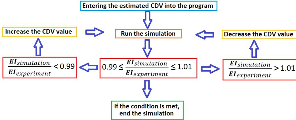
**Figure 5.** Schematic depiction of determining the CDV value in the simulations
