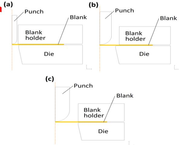
Figure 3. Simulation designs for the different die sets with Deform 2D; a)  $P_D = 8$  mm, b)  $P_D = 20$  mm, c)  $P_D = 25$  mm
