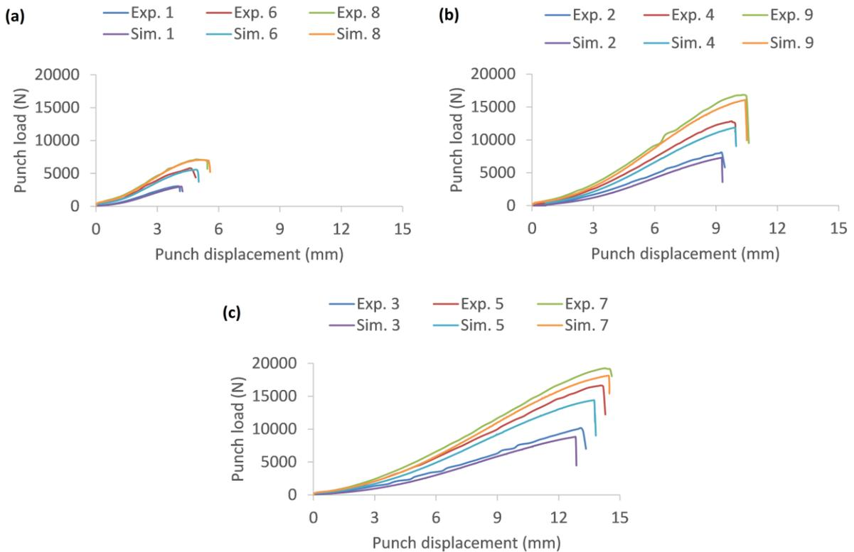
**Figure 20.** Displacement-punch force curves plotted using both experimental and simulation data of the DC04 steel sheets; a) the  $P_D = 8$  mm, b) the  $P_D = 20$  mm, c) the  $P_D = 25$  mm
