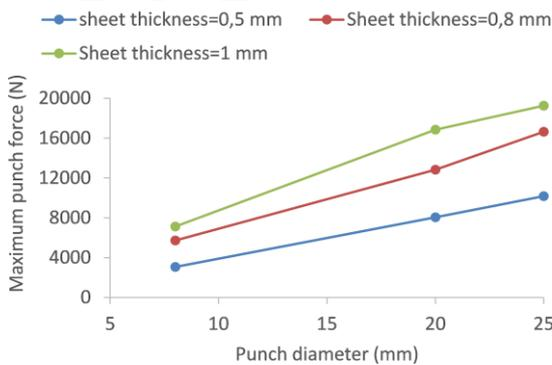
**Figure 13.** Impact of varying punch diameters on the maximum punch force
