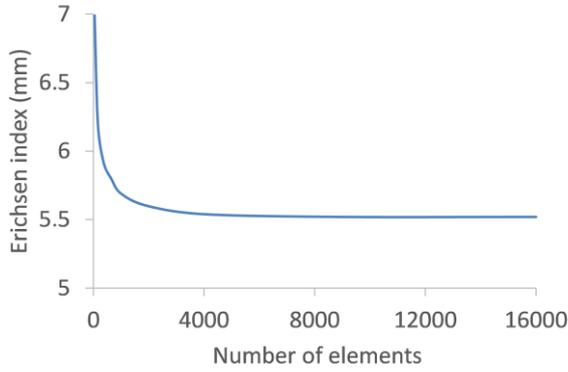
**Figure 4.** Dependence of the Erichsen index on the number of elements
