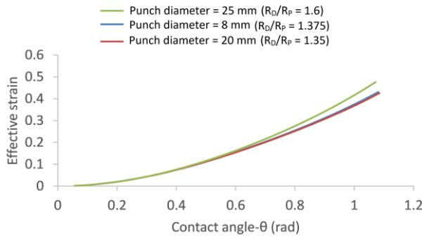
**Figure 18.** Variation of the effective strain ( $\bar{\epsilon}_e$ ) with the contact angle ( $\theta$ )
