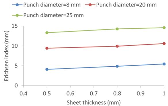
**Figure 19.** Variation of the Erichsen index with the sheet thicknesses
