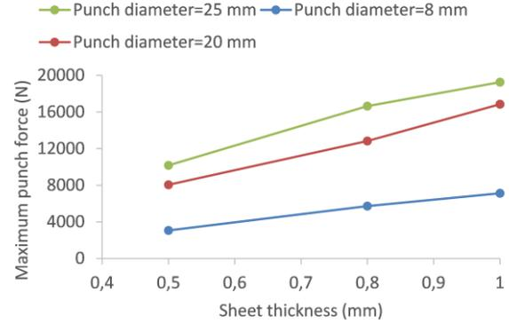
**Figure 14.** Impact of varying sheet thicknesses on the maximum punch force
