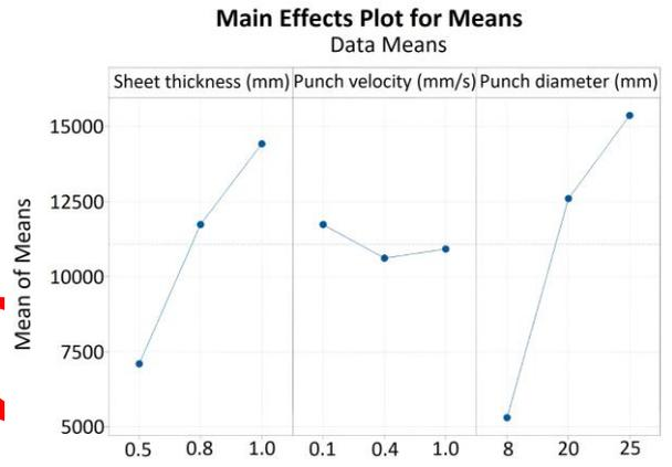
**Figure 11.** Means of maximum punch forces acquired via the Taguchi analysis
