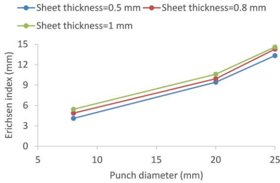
**Figure 17.** Variation of the Erichsen index with the punch diameters
