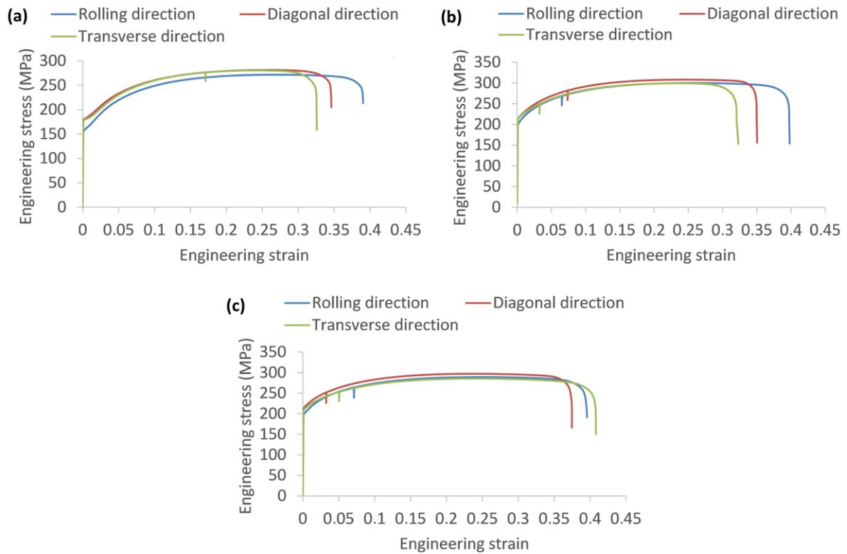
**Figure 6.** Engineering stress-strain curves of sheet materials; a) 0.5 mm DC04 sheet material, b) 0.8 mm DC04 sheet material, c) 1.0 mm DC04 sheet material
