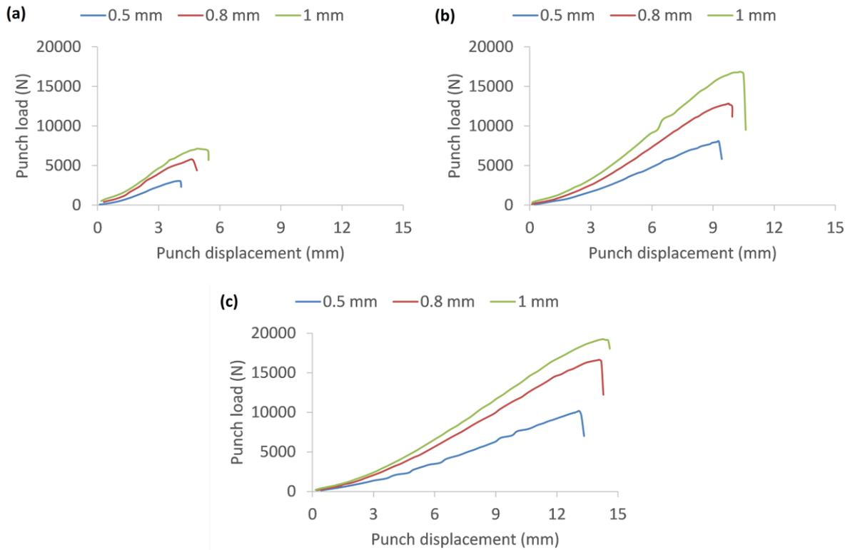
**Figure 7.** Displacement-Punch force curves of the DC04 steel sheets for various thicknesses; a) the  $P_D = 8$  mm, b) the  $P_D = 20$  mm, c) the  $P_D = 25$  mm
