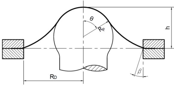
**Figure 12.** Deformation geometry during the Erichsen test
