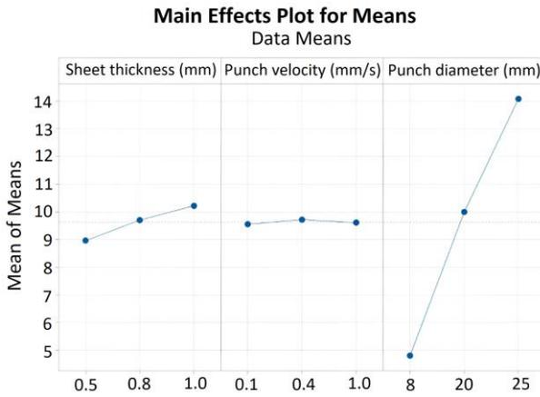
**Figure 9.** Means of EI values acquired via the Taguchi analysis
