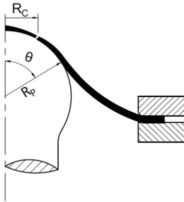
**Figure 22.** Schematic illustration of the crack formed during the Erichsen test.
