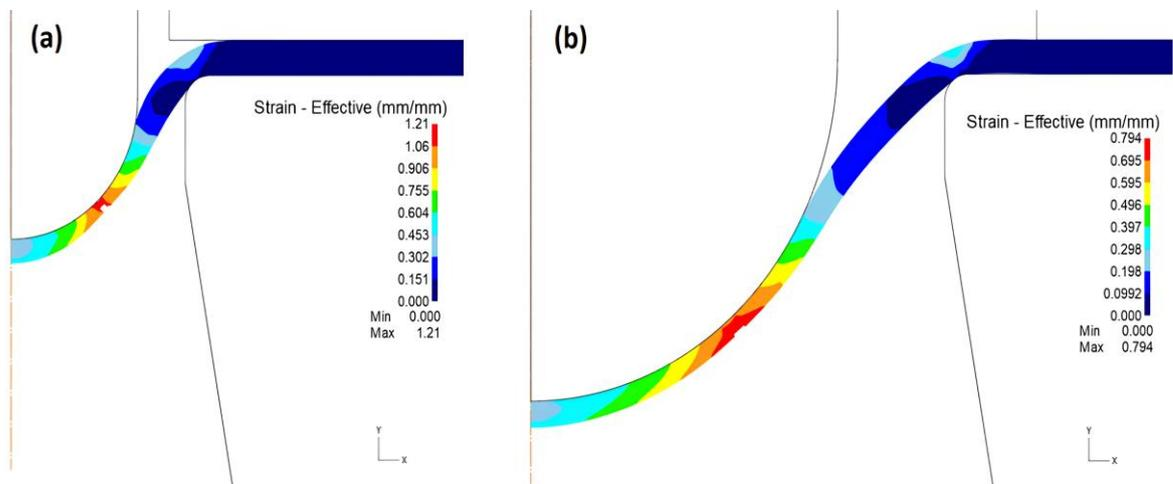
**Figure 23.** The effective strain values occurring in the DC04 steel sheet at the moment the crack initiates; a) the  $P_D = 8$  mm, b) the  $P_D = 20$  mm
