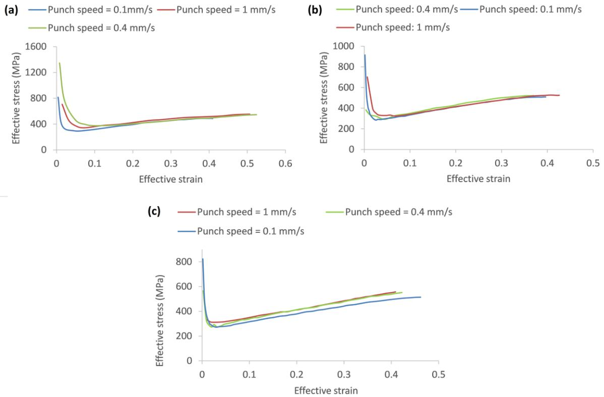
**Figure 15.** Stress-strain curves obtained at different punch speeds from the Erichsen experiments; a) the  $P_D = 8$  mm, b) the  $P_D = 20$  mm, c) the  $P_D = 25$  mm
