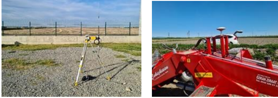
Figure 3. Reference station and GPS receiver
