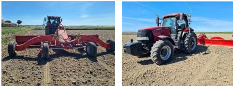
Figure 4. Leveling shovel with GPS leveling system
