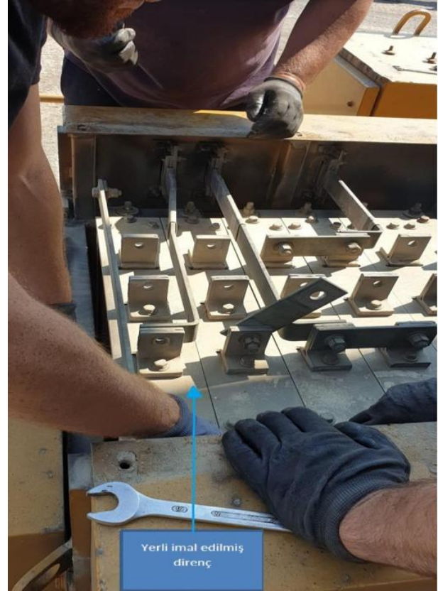
Figure 3. Installation of locally produced resistor
