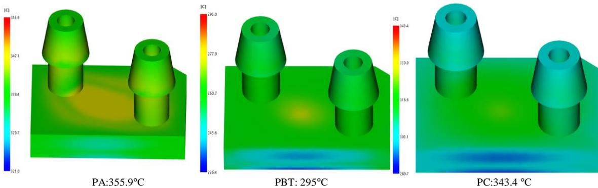
Fig. 14. Bulk temperature at end of fill results.
