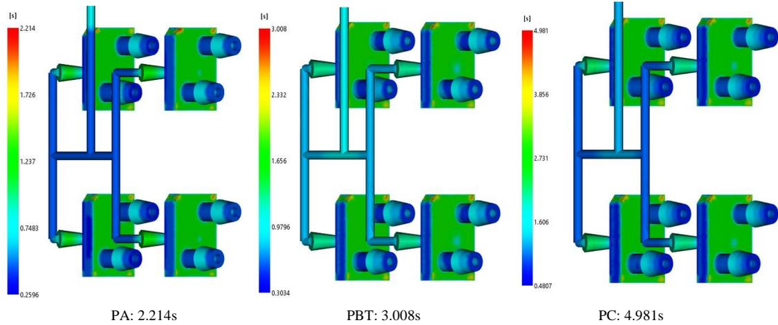
Fig. 13. Time to reach ejection temperature results.
