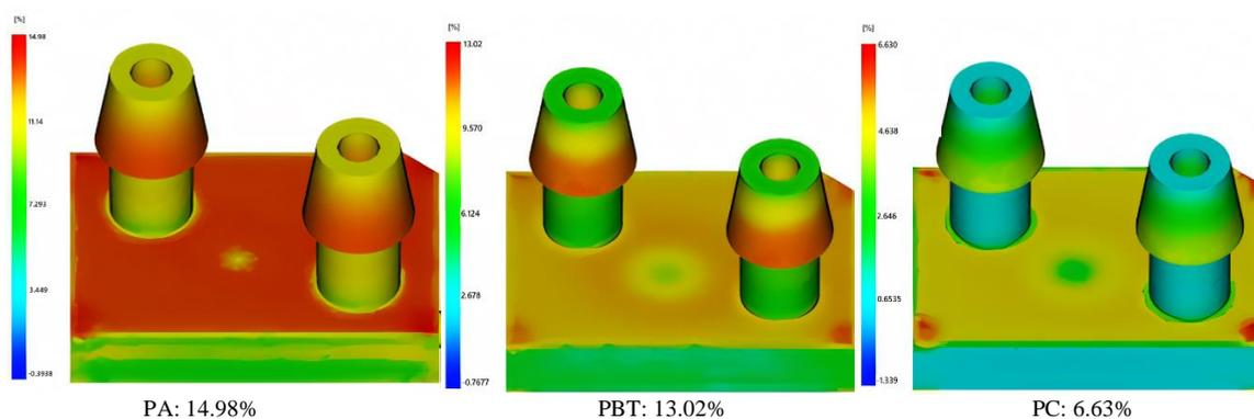
Fig. 12. Volumetric shrinkage values.
