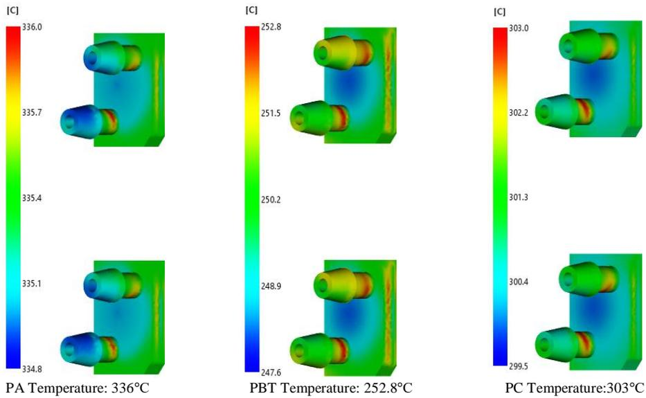
Fig. 10. Temperature at front flow analysis results.
