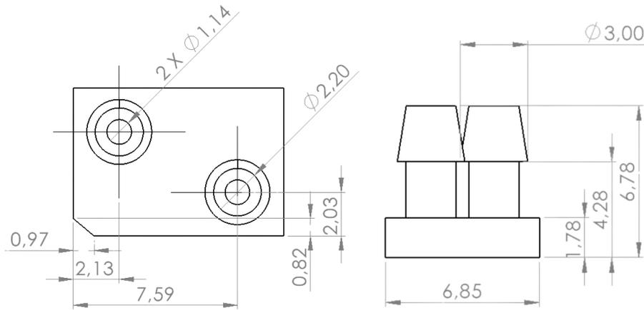
Fig. 1. Technical drawing dimensions of the model.
