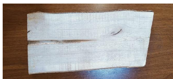
Figure 2. The direction of the cavity in a radial section of wood
