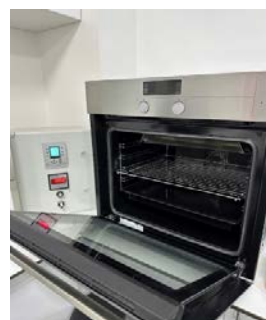
Figure 1. Designed infrared oven used in the experiments
