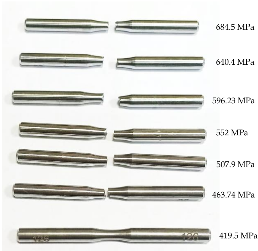
Figure 14. Fractured and unfractured AISI 304 stainless steel specimens after the fatigue test and stress values applied to these specimens.
