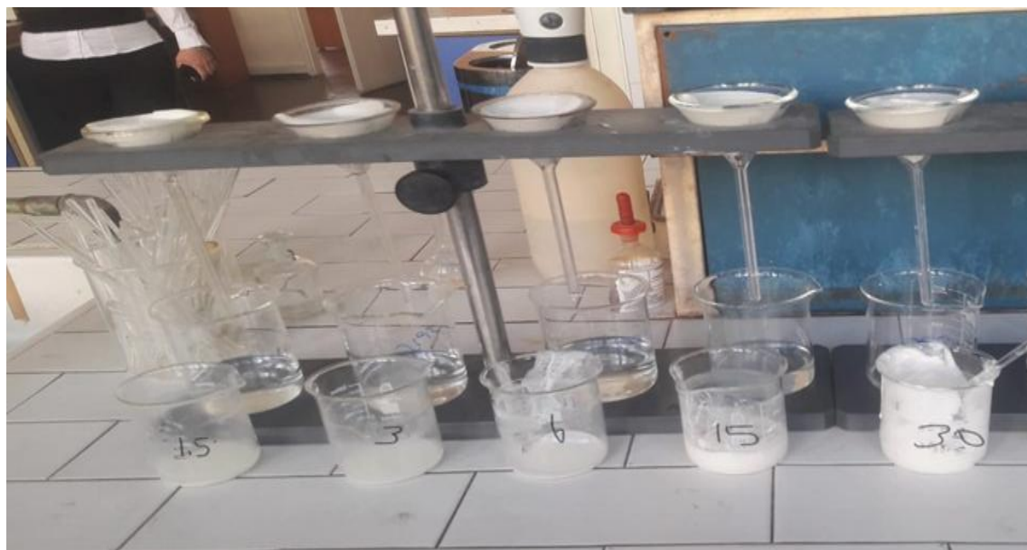
Figure 4. Filtration After Chemical Precipitation with Different Amounts of Lime at 55 °C
