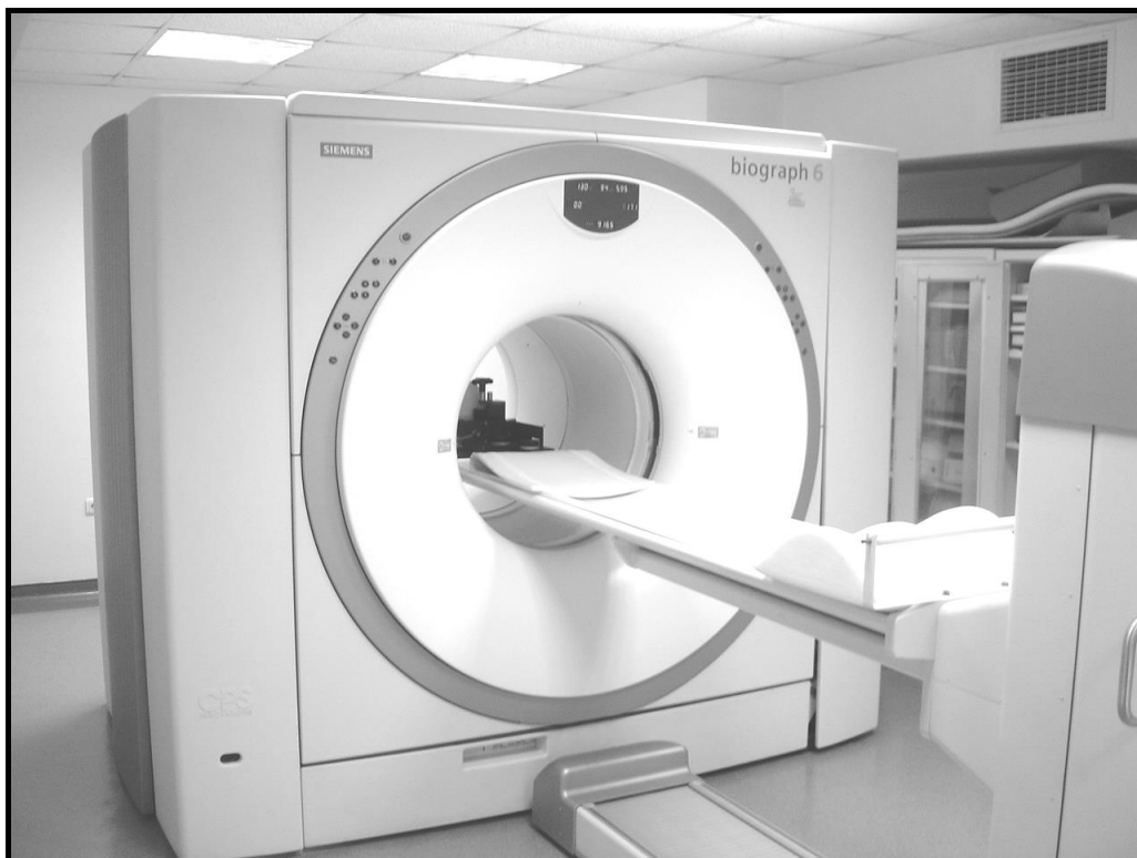
Figure 4: The CT scanner consists of a fast ceramic detector with the ability to acquire 6 slices.
