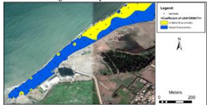
Fig. 20. Map of spatial variation in the coefficient of uniformity for khaloufi beach.
