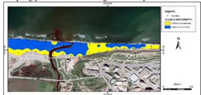
Fig. 21. Map of spatial variation in the coefficient of uniformity for corso beach.
