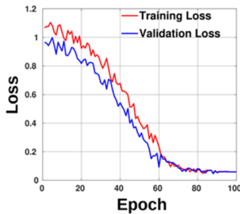
Figure 5. The proposed model was trained for 100 epochs for optimizing the mean squared error loss function with rmsprop. A dynamic learning rate scheduler is used. After 100 epochs the loss curves reached saturation. The model is trained with Tensorflow framework using four RTX-A6000 GPUs.
