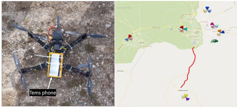
Figure 1. TEMS phone, Ground control station interface and UAV route
