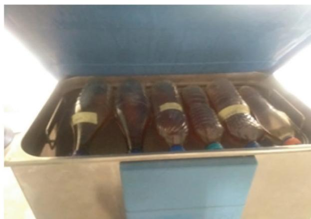
**Figure 2.** Pictorial view of blends in the ultrasonicator.
