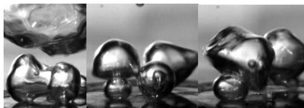
Figure 13. Events of bubbles merging in the vicinity of the boiling surface in horizontal, vertical, and diagonal axes [28].
