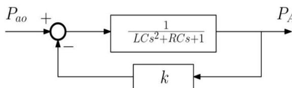
**Figure 4.** Proportional feedback of the ventilator system [1].
