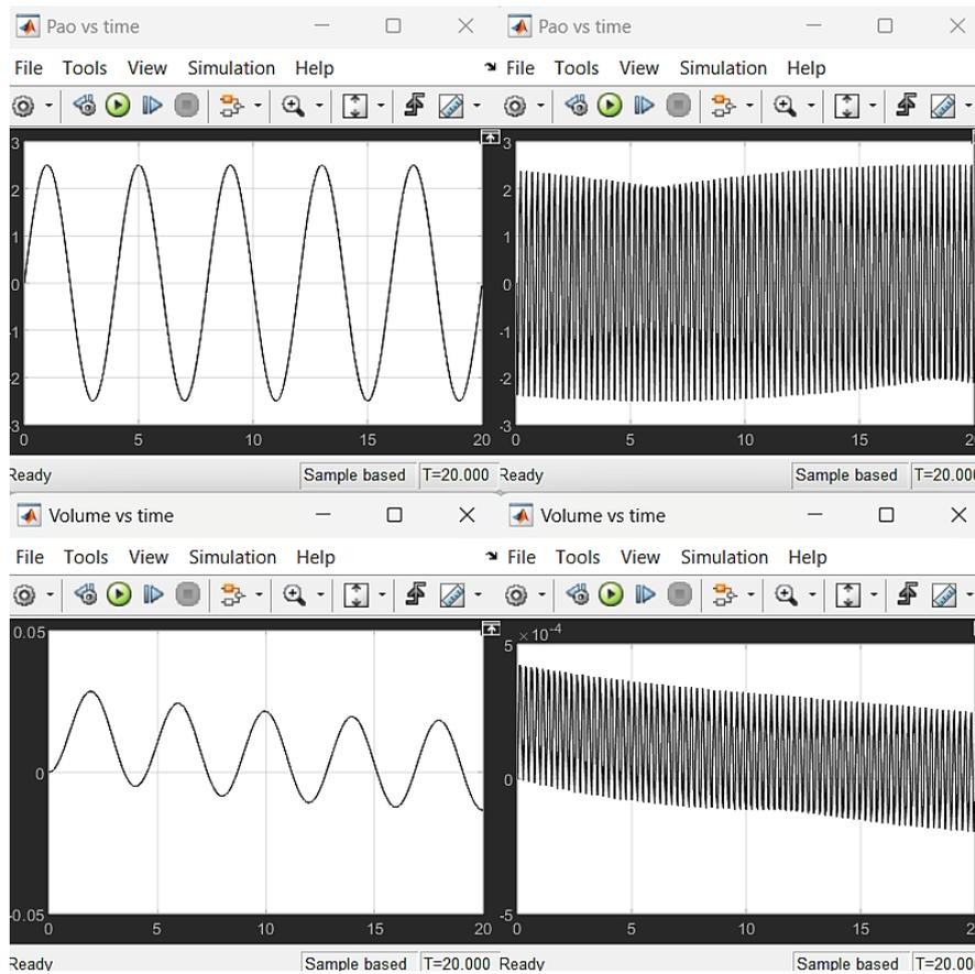
**Figure 5.** Pressure at the airway opening and volume graphs (from up to down) with proportional feedback effect for 15 and 960  $breaths\ min^{-1}$  (from left to right), respectively.
