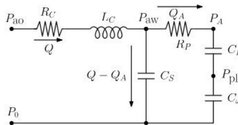
**Figure 1.** Circuit design representation of the linear model. The quantity  $P_0=0$ .
