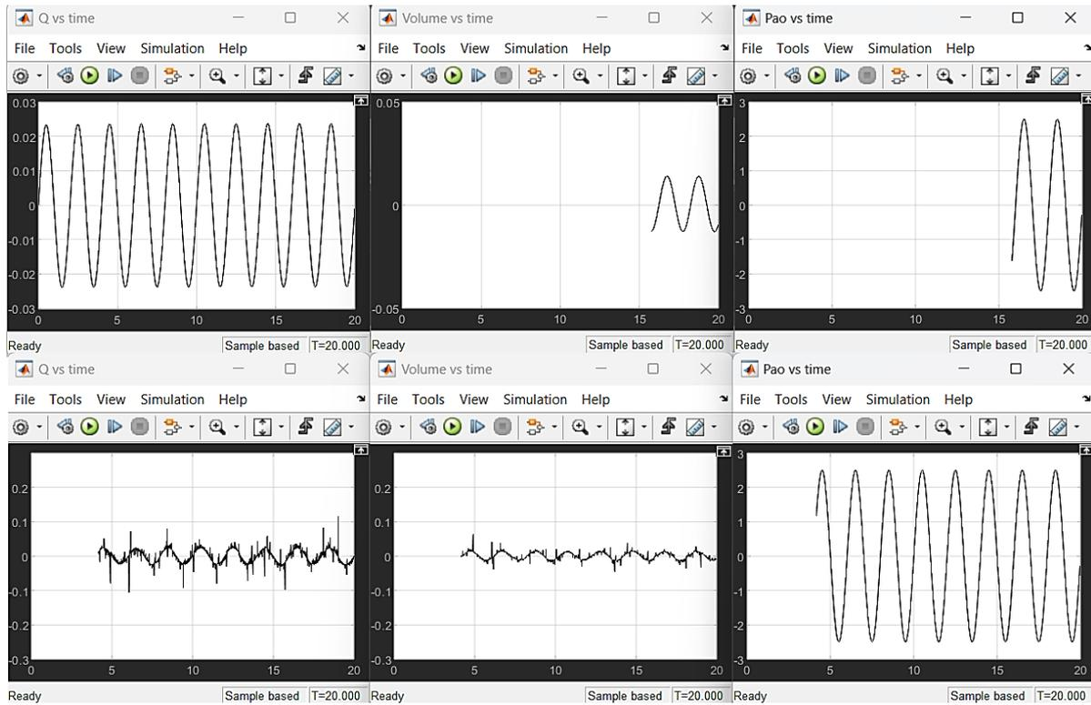
**Figure 7.** Air flow, tidal volume, pressure at the airway opening graphs of  $30 \text{ breaths min}^{-1}$  for a healthy individual (up) and a patient with esophageal balloon (bottom) when fractional-order derivative 0.5 is used.
