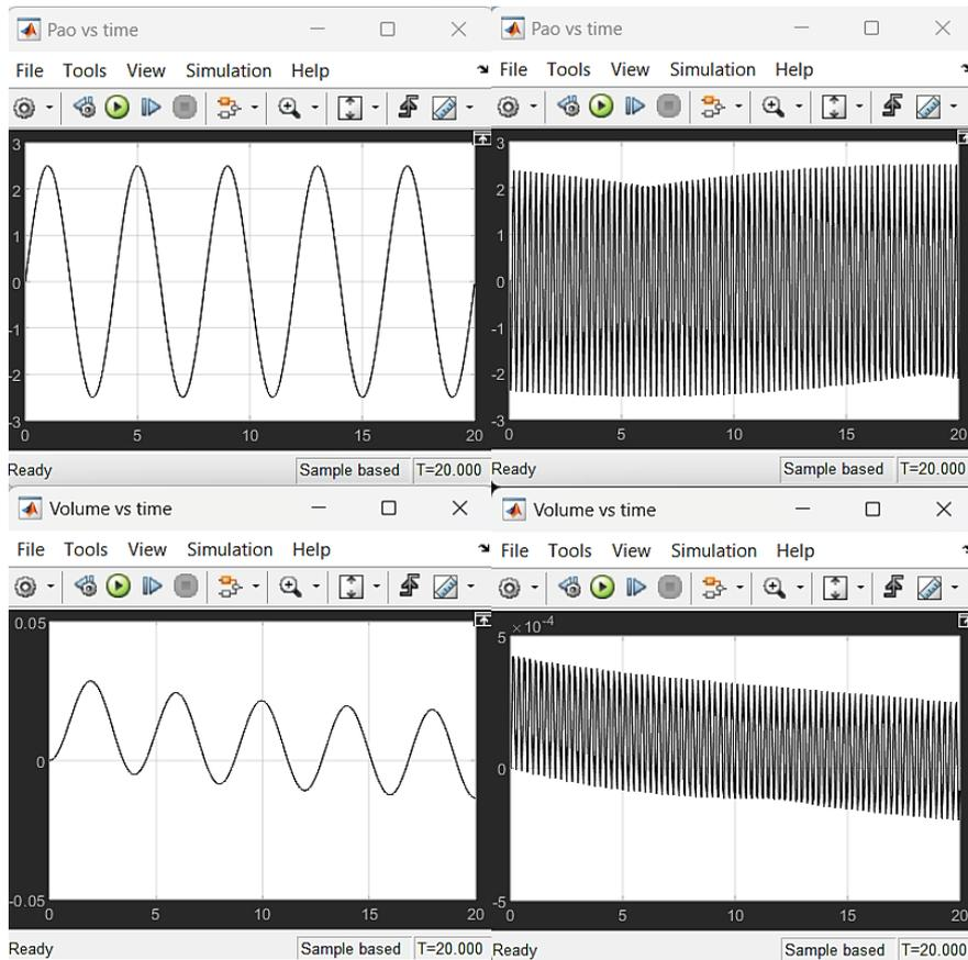
**Figure 3.** Pressure at the airway opening and volume graphs (from up to down) without proportional feedback effect for 15 and 960  $breaths \text{ min}^{-1}$  (from left to right), respectively.
