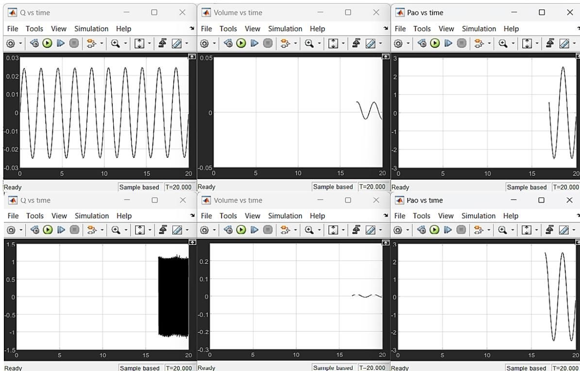
**Figure 6.** Air flow, tidal volume, pressure at the airway opening graphs of 30  $breaths\ min^{-1}$  for a healthy individual (up) and a patient with esophageal balloon (bottom) when integer order derivative is used.
