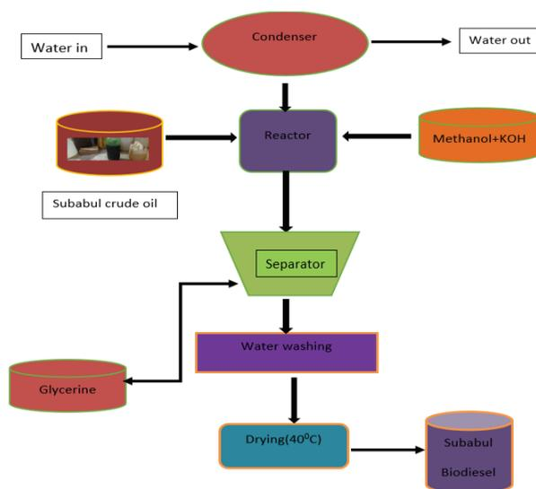
Figure 1. Biodiesel production through transesterification method.
