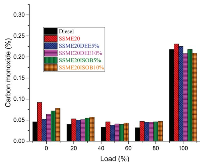
Figure 8. Carbon monoxide emissions variation with engine load.
