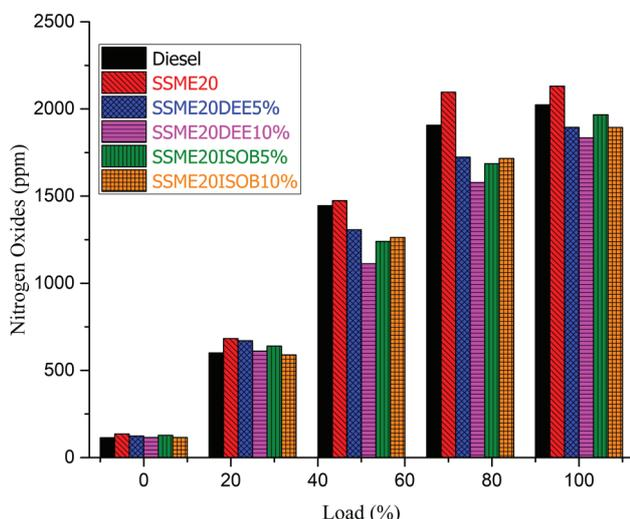
Figure 9. NOx emissions variation with engine load.
