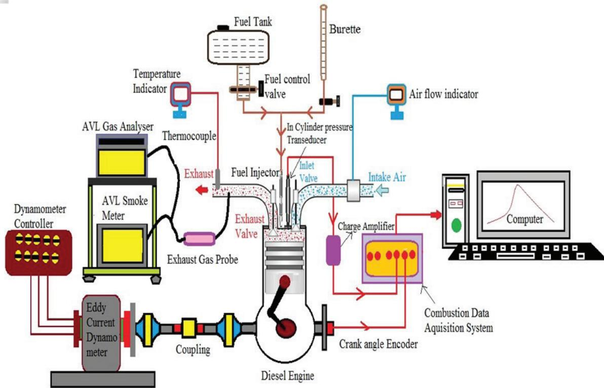
Figure 2. Schematic view of experimental engine setup.
