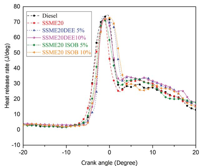
**Figure 6.** Variation of HRR with crank angle.
