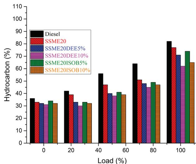
Figure 7. HC emission variation with engine load.
