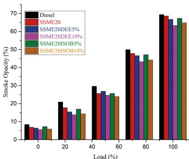
Figure 10. Smoke opacity variation with engine load.
