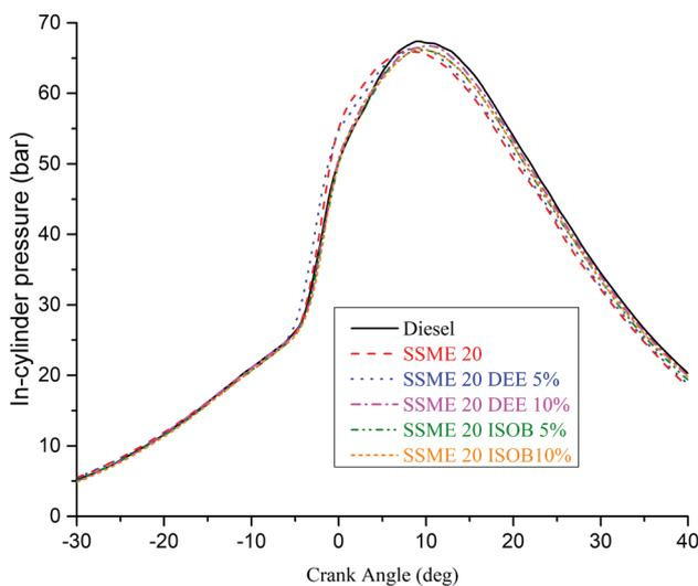
**Figure 5.** In-cylinder pressure variation with crank angle.
