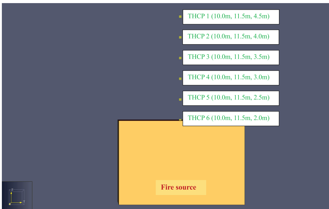
Figure 12. Arrangement of thermocouples.
