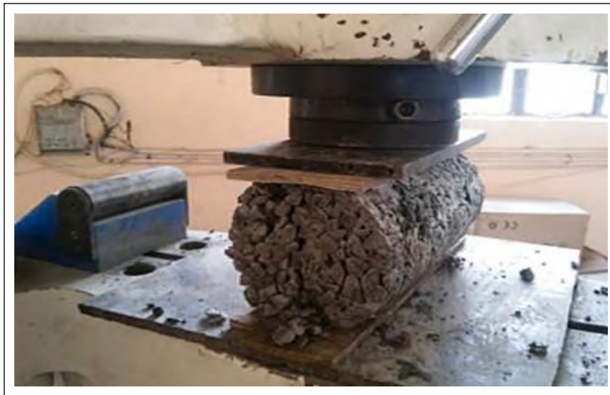
Figure 9. Tensile strength determination using the Brazilian approach.
