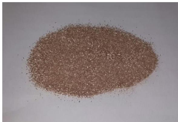
Fig. 2. Vermiculite (Super Fine) used in Experiments
