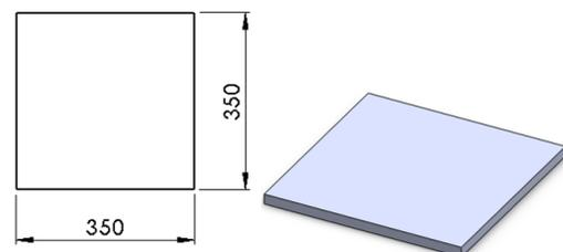
Figure 4. Technical drawing and solid model view of the table part
