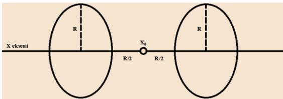
Figure 1. Schematic representation of the Helmholtz coil [5]
