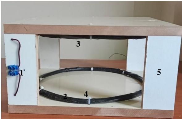
Figure 6. Manufactured EMF generator
