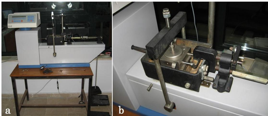
**Figure 4.** Shear strength test: a) Shear test machine, b) a view of shear box part of the machine
