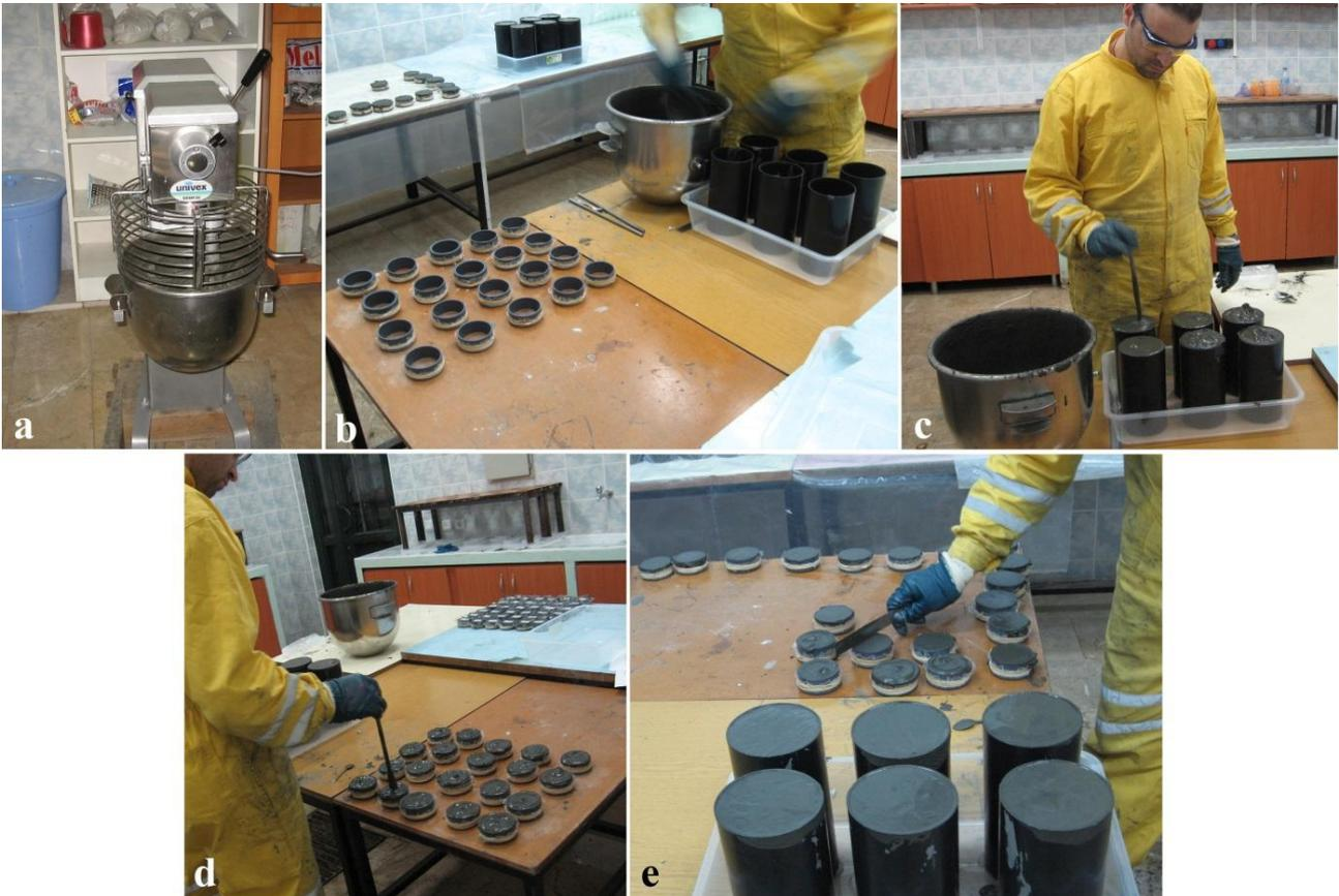
Figure 2. Specimen preparation: a) mixing, b) molding, c and d) compaction with the tamping rods, e) surface flattening
