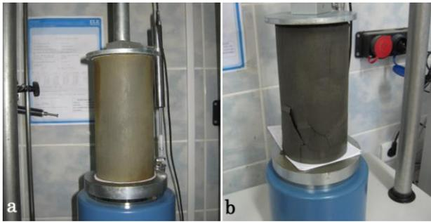
**Figure 3.** UCS test: a) a specimen under load, b) a failed specimen
