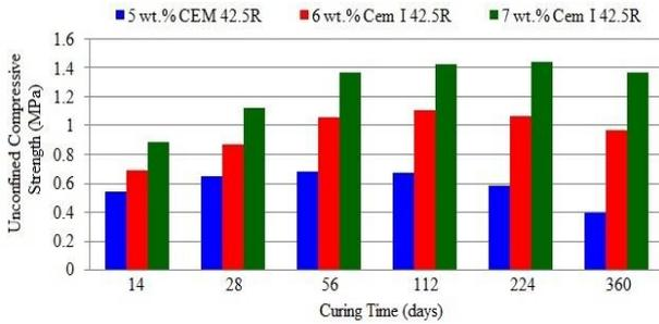
**Figure 5.** UCS values for different curing time and cement contents
