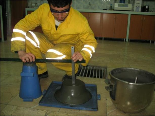
Figure 1. Slump test for CPB mixes
