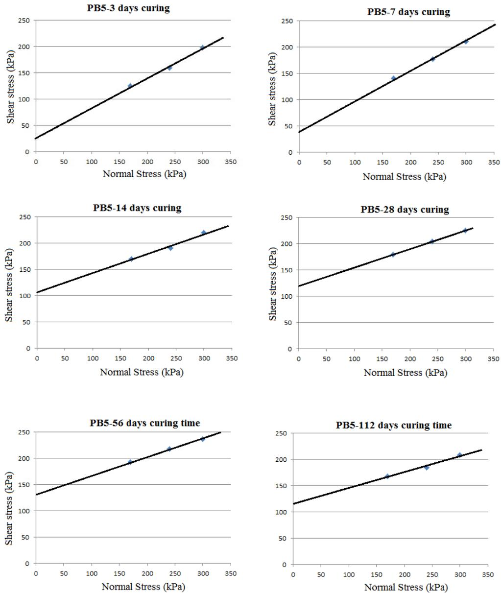
**Figure 7.** Some examples for shear strength variations under different normal stress conditions
