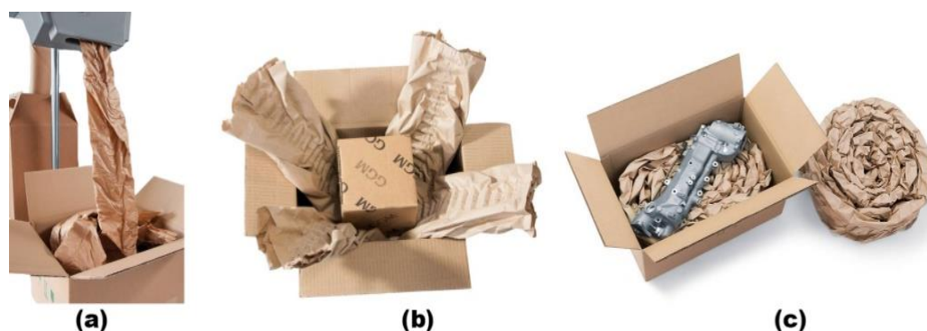
Figure 2. Buffering operations: a). Forming machine used to increase the flexibility of the material such as paper newspaper to be used in the buffering process. b) Filling the space in the primary packaging in the transport package to prevent external impact and possible vibration. c) The buffering process by filling the packaging space in the primary packaging to protect the product directly
