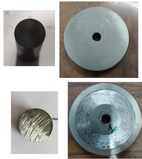
Figure 5: Pin & Disk a) Before test b) After test
