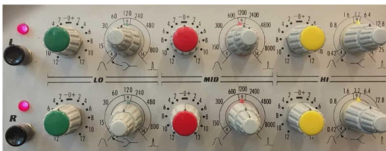
Photo 2. The first parametric equalizer developed by Burgess MacNeal and George Massenburg. ITI Audio MEP-130 Console EQ-1969 (Web 2)
