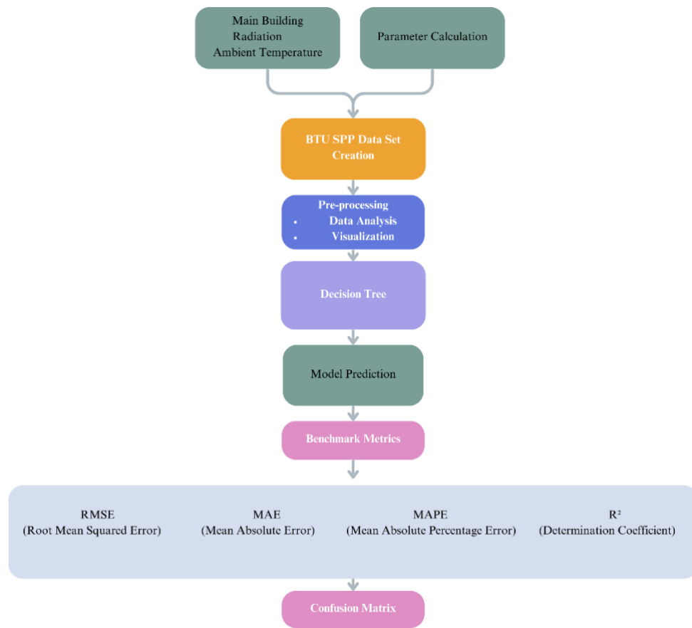
Figure 7: BTU G Block Electric Power Generation Prediction Flowchart
