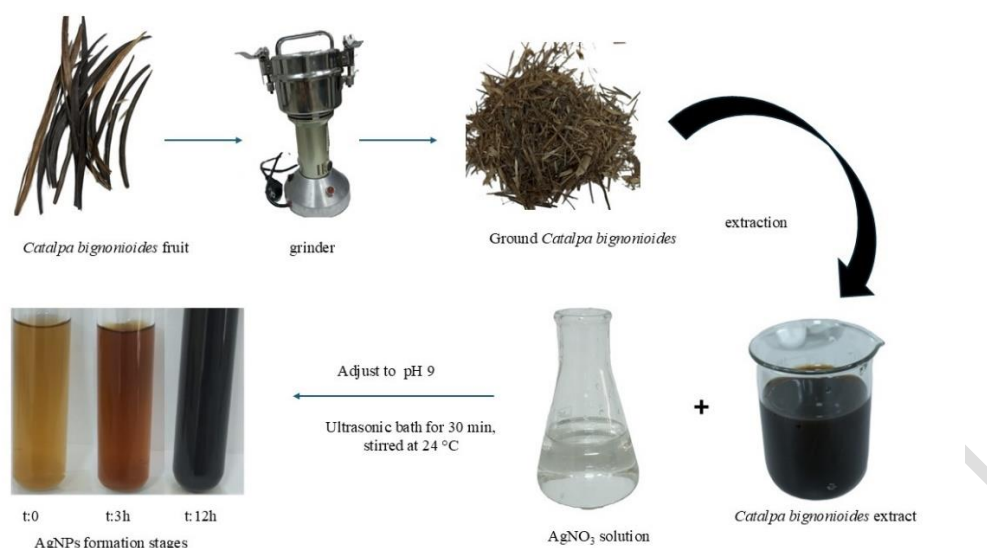
Figure 1. AgNPs synthesis steps using FCB.
