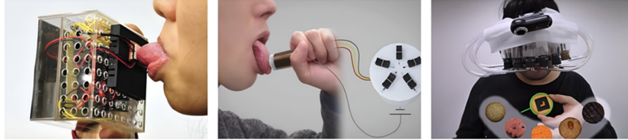
Figure 7. VR taste simulators [63].
