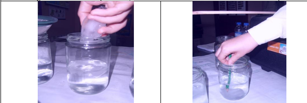
Stage 4. A large piece of ice is thrown in the third jar and it is pushed to the bottom with the help of a pen or a stick. The level is measured when the ice is under the water.
