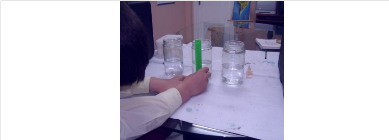
Stage 3. Pieces of ice are put in the jar and its level is measured and recorded immediately
