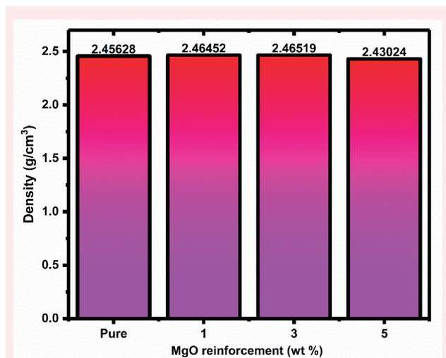
**Figure 3.** Density Analysis of Al-Cu Composites Reinforced with Varying MgO Percentages
