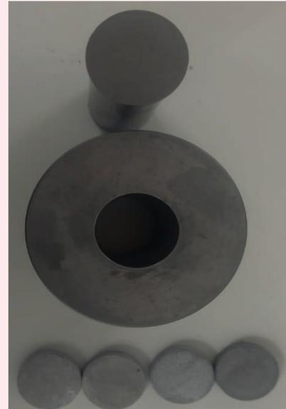
Figure 1. The press die having 3 cm diameter and bulk samples of Al-Cu composite
