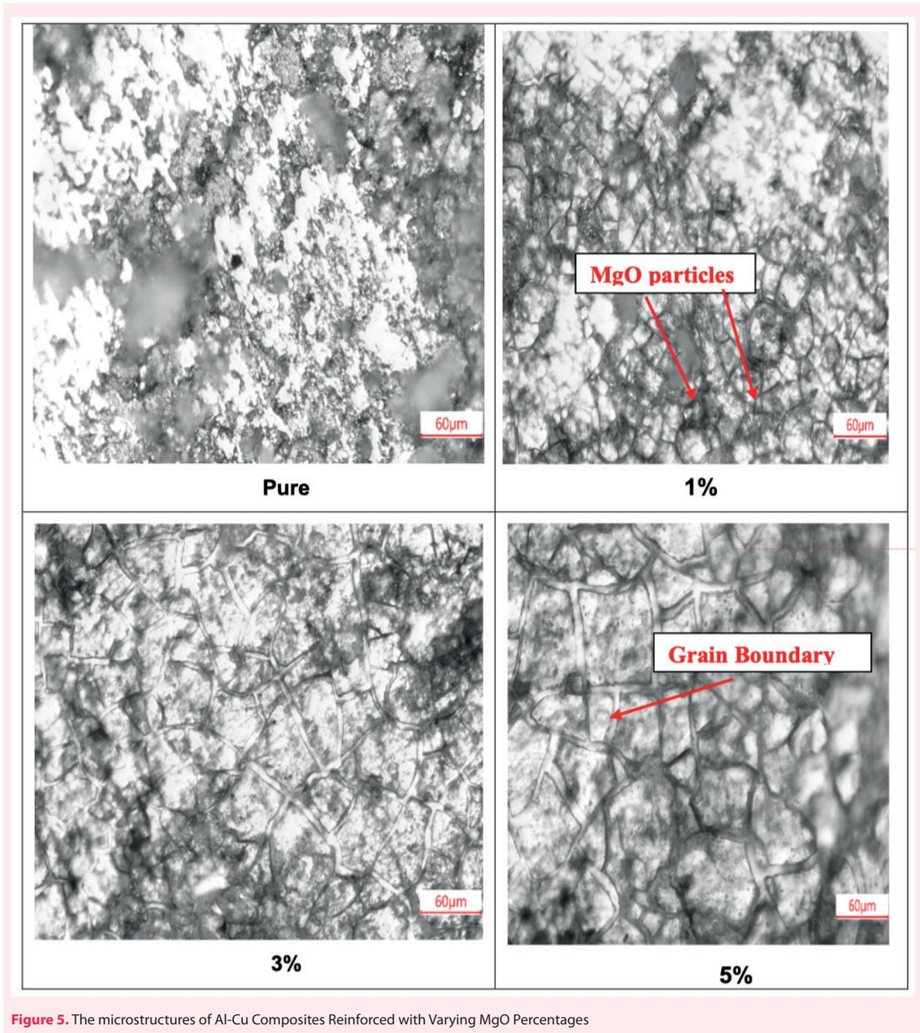
Figure 5. The microstructures of Al-Cu Composites Reinforced with Varying MgO Percentages
