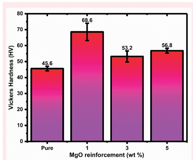
**Figure 4.** Hardness Analysis of Al-Cu Composites Reinforced with Varying MgO Percentages
