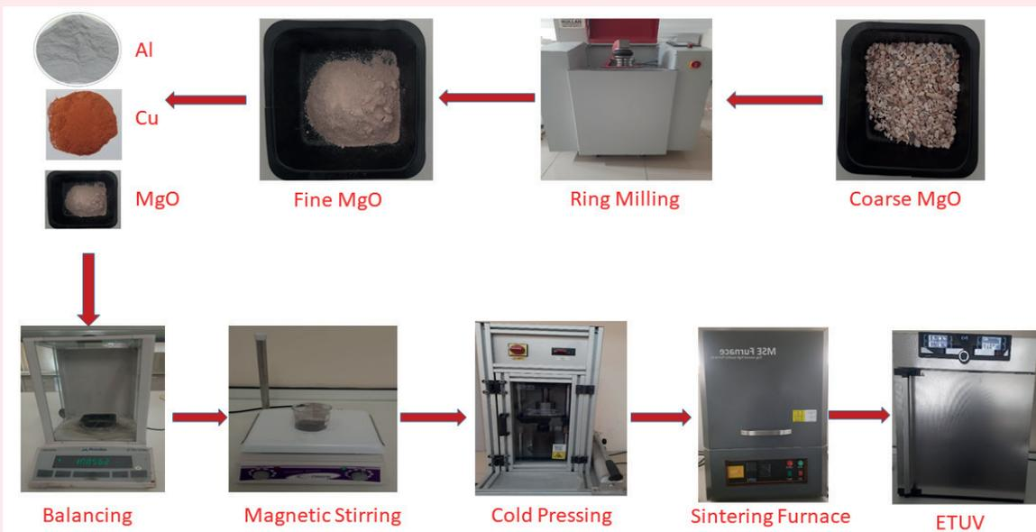
Figure 2. The procedure for producing MgO reinforced Al-Cu composites
