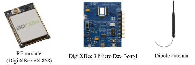
Figure 2. The main components of T_x and R_x nodes.
