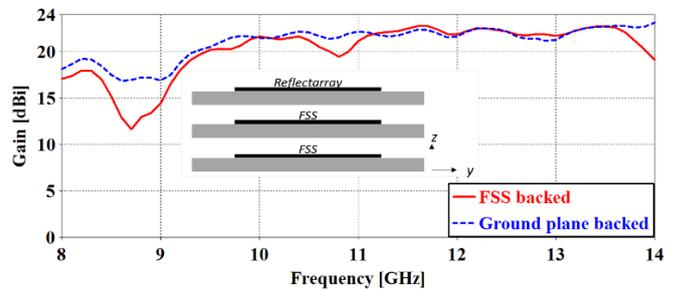
Figure 8. Gain curves for the ground plane backed reflectarray antenna and FSS backed reflectarray antenna.
