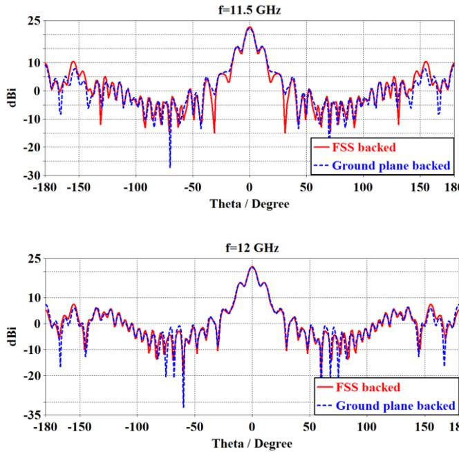
**Figure 9.** Radiation patterns of FSS backed and ground plane backed reflectarray antenna at 11.5 GHz and 12 GHz ( $\phi=90^\circ$ ).
