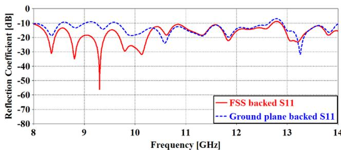
Figure 6. S<sub>11</sub> parameter of reflectarray antenna with ground plane backed and FSS backed.
