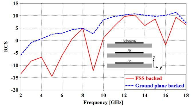
Figure 7. Relationship between the monostatic RCS levels of the ground plane backed and FSS backed reflectarray antennas.
