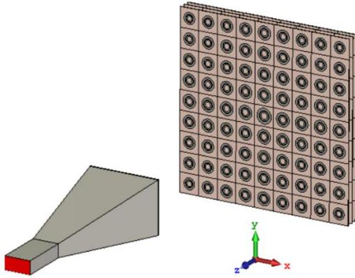
Figure 4. Reflectarray antenna with FSS backed.
