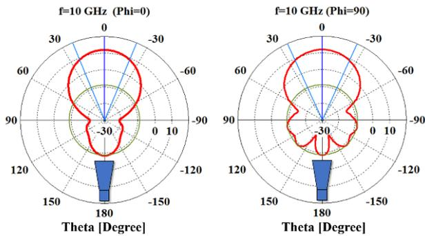
Figure 5. Simulated radiation patterns of horn antenna at 10 GHz for E-plane and H-plane.
