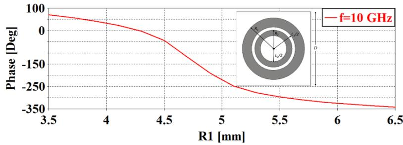
Figure 2. Reflection phase curve of the unit cell.
