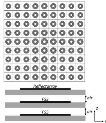
Figure 3. Reflectarray structure and double-layer settlement behind the reflectarray antenna used for FSS layer.
