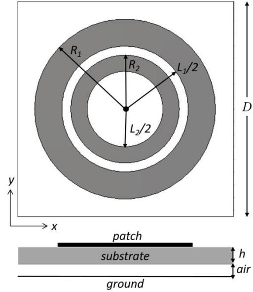
Figure 1. The view of reflectarray unit cell.
