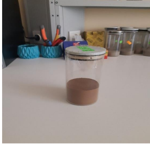
Fig. 2. Cylindrical container in which LR-115 is placed.
