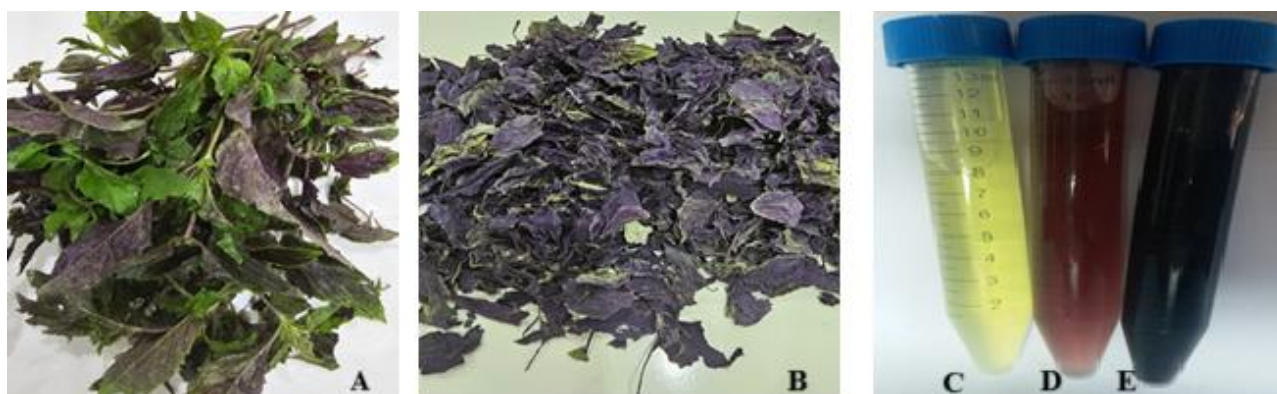
Figure 1. A. Fresh leaves of OB. B. Dried leaves. C. \text{HAuCl}_4 \cdot 3\text{H}_2\text{O} solution (Yellow). D. OB aqueous extract (Red). E. Biosynthesized OB-AuNPs solution (Dark red)
