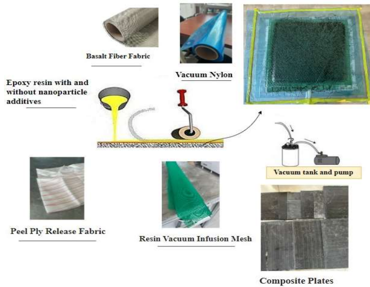
Figure 3. Production of composite plates using hand lay-up + vacuum bagging method
