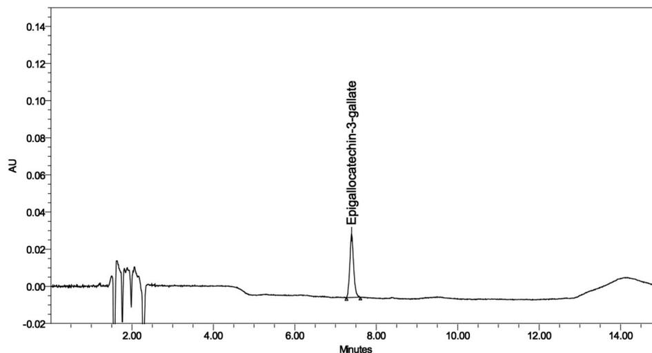
Figure 2. Chromatogram of standard epigallocatechin 3 gallate at LQC level (5µg/ml) spiked in rat plasma. (Rt = 7.417 minutes)
