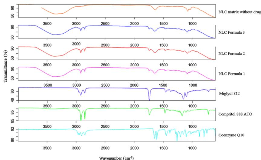
**Figure 1.** Infrared spectra of Coenzyme Q10, Compritol 888 ATO, Miglyol 812, NLC Formula 1, NLC Formula 2, NLC Formula 3, and NLC matrix at wave numbers 400-4000  $\text{cm}^{-1}$
