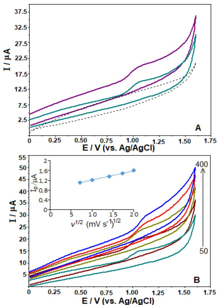
**Figure 1.** Performance of CVs for  $100 \mu\text{g mL}^{-1}$  NFX in BR buffer solution (pH 6.0) on the BDD electrode at the scan rate of  $100 \text{ mV s}^{-1}$  (A), and CVs undergo analysis at various scan rates, including 50, 100, 200, 300 and  $400 \text{ mV s}^{-1}$ . The background current is visually represented using dashed lines (A). The plots of  $I_p$  versus  $v^{1/2}$  are included as insets (B).
