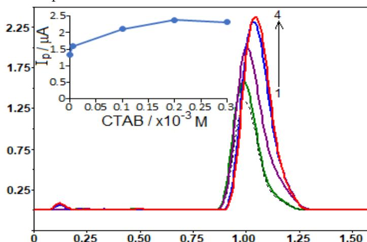
**Figure 5.** SW voltammograms of  $0.75 \mu\text{g mL}^{-1}$  NFX in the solution of BR buffer at pH 6.0 with the existence of different CTAB concentrations (from 1 to 4;  $5.0 \times 10^{-5} - 3 \times 10^{-4} \text{ M}$ ) at the CPT-BDD electrode. Dashed lines depict the voltammograms obtained without CTAB. Inset: a graph of  $I_p$  versus CTAB concentration. SWV parameters; step potential, 16 mV; pulse amplitude, 50 mV; frequency, 100 Hz.
