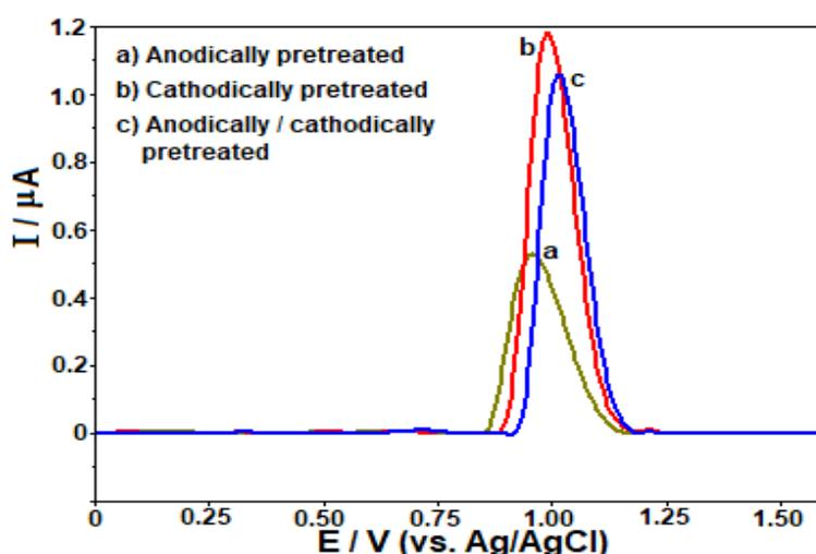
**Figure 2.** Recorded in BR buffer solution (pH 6.0) using the BDD electrode after various electrochemical pretreatments, the SW voltammogram shows 2  $\mu\text{g mL}^{-1}$  NFX. The SWV parameters were as follows: step potential, 10 mV pulse amplitude, 40 mV; frequency, 50 Hz.
