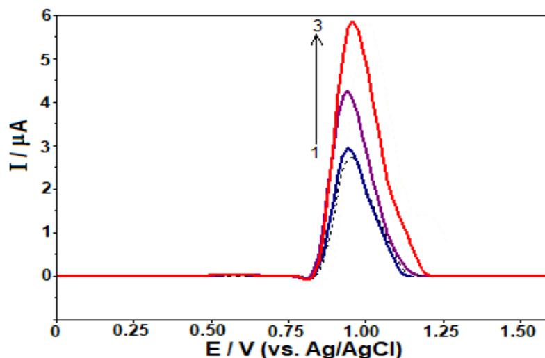
**Figure 7.** SW voltammograms of the diluted capsule sample (dashed line) and after standard additions of 0.1, 0.5, and 1.0  $\mu\text{g mL}^{-1}$  NFX (1-3) in BR buffer solution at pH 6.0 with  $2 \times 10^{-4}$  M CTAB on the CPT-BDD electrode. Other working situation are illustrated in Figure 6.
