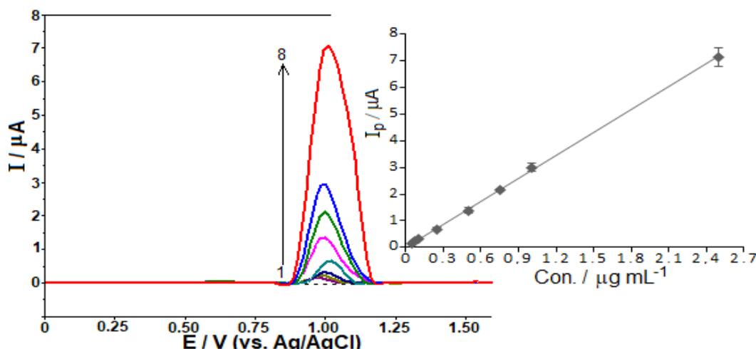
**Figure 6.** SW voltammograms for NFX levels of (1-8) 0.05, 0.075, 0.10, 0.25, 0.50, 0.75, 1.0 and 2.5  $\mu\text{g mL}^{-1}$  in the solution of BR buffer at pH 6.0 with  $2 \times 10^{-4}$  M CTAB. Other working situation are illustrated in Figure 5.
