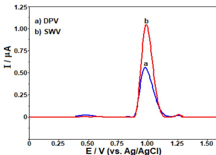
**Figure 4.** DP (a) and SW (b) voltammograms of  $2 \mu\text{g mL}^{-1}$  NFX in BR buffer solution (pH 6.0) at the CPT-BDD electrode. DPV parameters: modulation time 0.05 s; step potential, 8 mV and modulation amplitude, 50 mV. Other working situation are illustrated in Figure 3.
