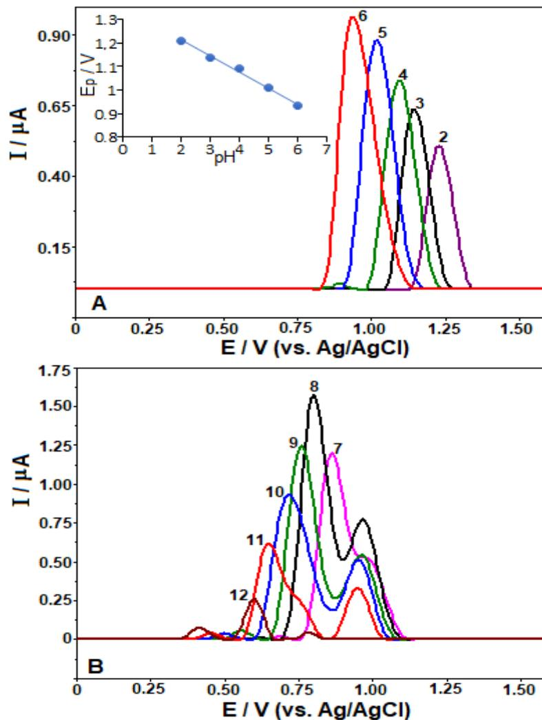
**Figure 3.** SW voltammograms in BR buffer for  $2 \mu\text{g mL}^{-1}$  NFX between pH 2.0-6.0 (A), and between pH 7.0-12.0 (B) at the CPT-BDD electrode. Other working situation are illustrated in Figure 2.
