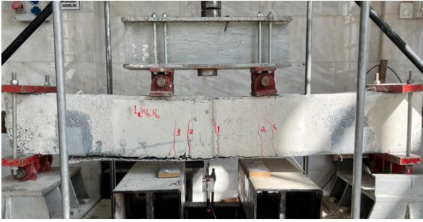
Figure 15. Appearance of L1W10H10 collapsed sample after three-point bending test
