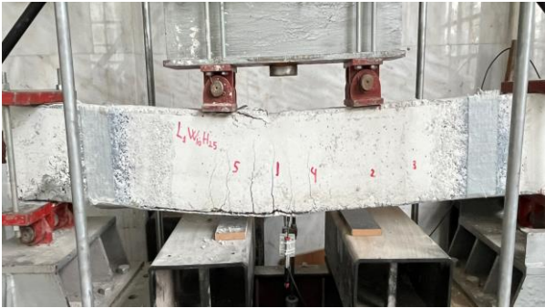
Figure 16. Appearance of L1W10H25 collapsed sample after three-point bending test
