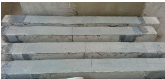
Figure 11. Examples of RC retrofitted beams with GFRP plates and anchors
