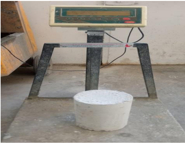
Figure 3. Concrete density test
