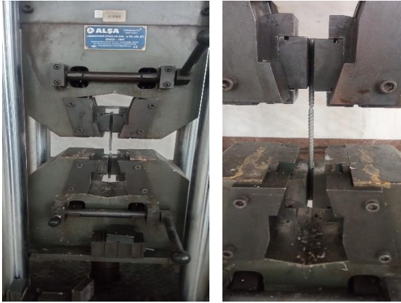
Figure 6. Tensile strength test of steel reinforcement
