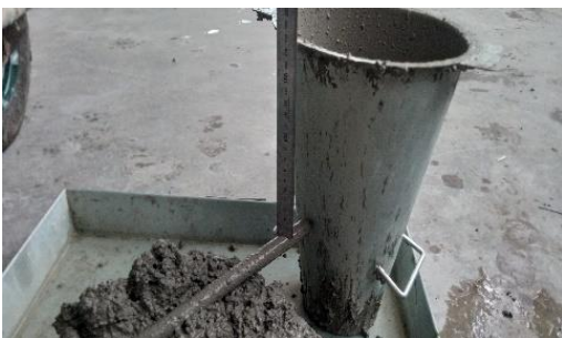
Figure 4. Slump test of cast in place concrete
