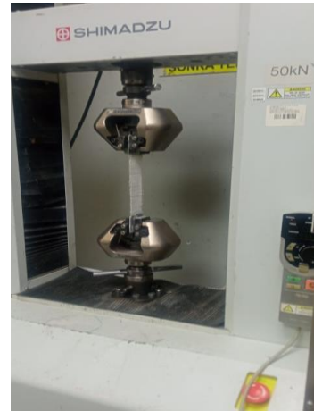
Figure 9. Tensile test of GFRP samples
