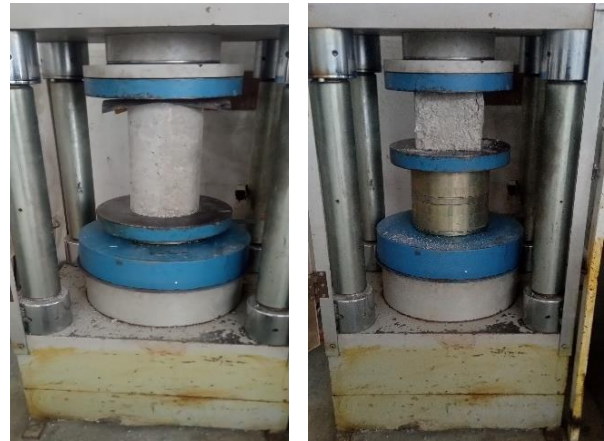
Figure 5. Compressive strength test of concrete samples
