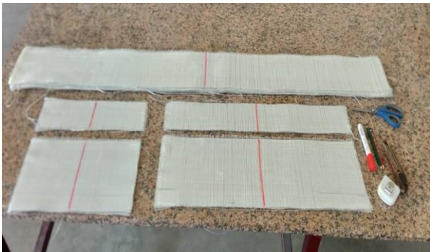
Figure 7. One-way oriented polymer reinforced fiberglass textile plates
