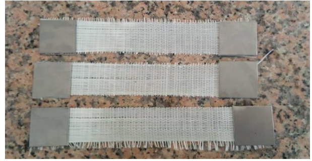
Figure 8. Tensile tested of GFRP samples
