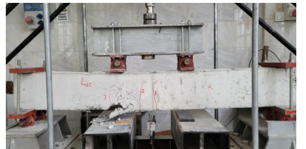
Figure 14. Appearance of L1C collapsed sample after three-point bending test
