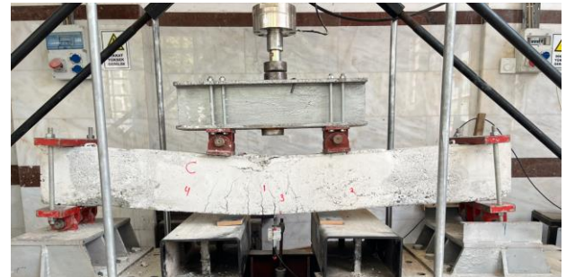
Figure 13. Appearance of C collapsed sample after three-point bending test
