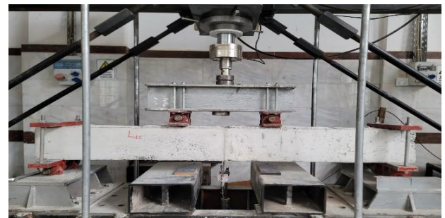
Figure 12. The machine of applied load on the tested beams
