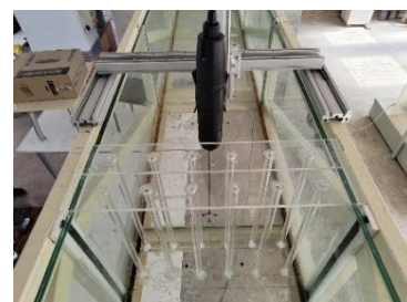
Six bridge piers of circular geometry placed along a double axis (Model 8)
