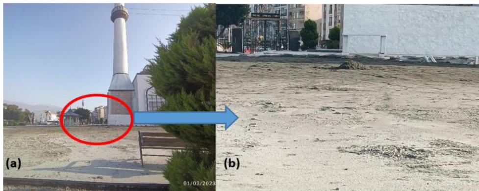
Figure 1. Surface ejecta observed around the close to İskenderun Bay during the first main Kahramanmaraş earthquake event
