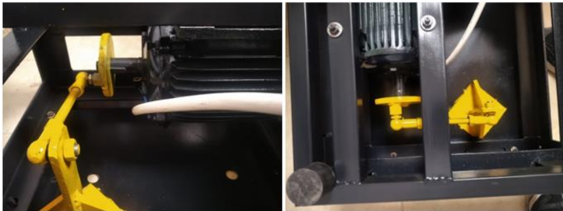
Figure 11. Mechanism used to convert circular motion into linear motion
