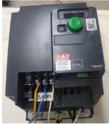
Figure 5. Used variable frequency drive
