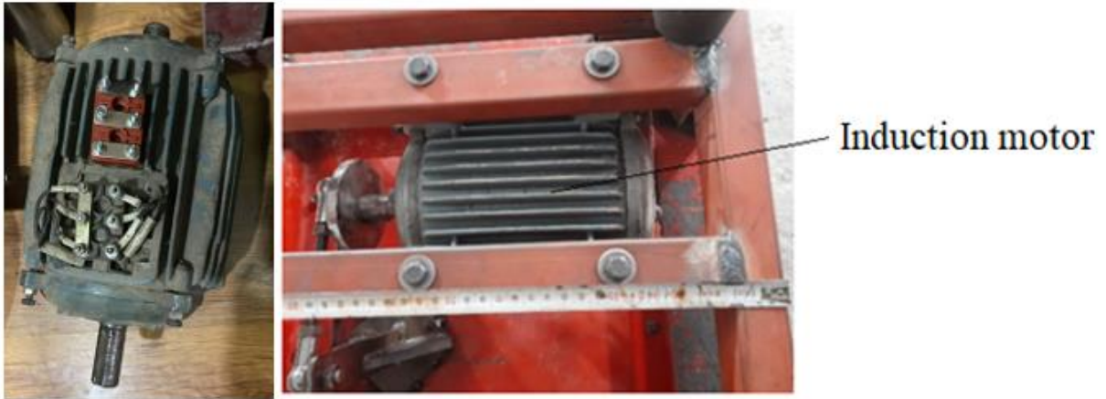
Figure 3. Induction motor obtained from scrap
