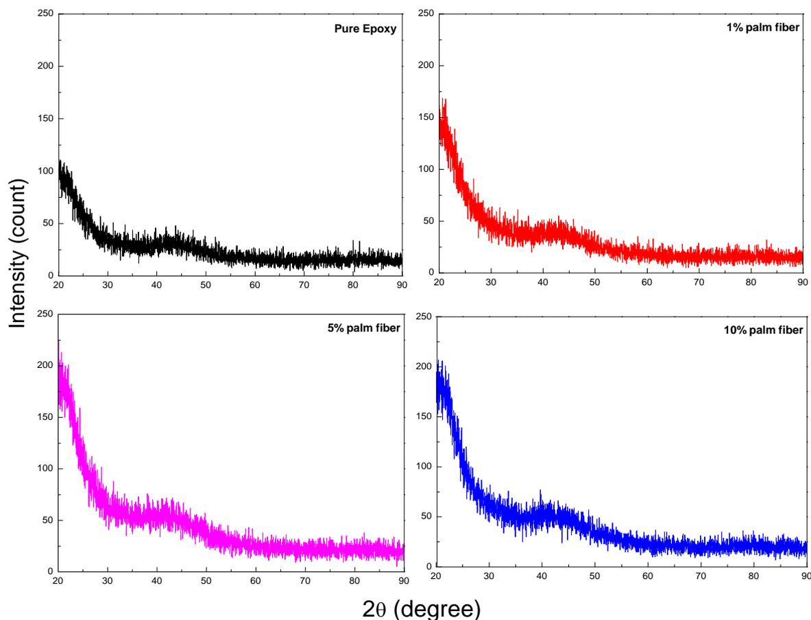
**Figure 2** XRD spectra of palm fiber reinforced epoxy eco composites
