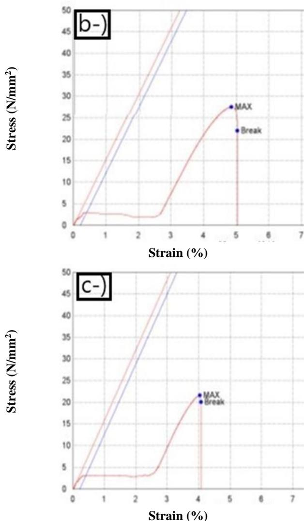
**Figure 1** Stress-strain graphs of 1% b-) 5% c-) 10% palm fiber reinforced composites
