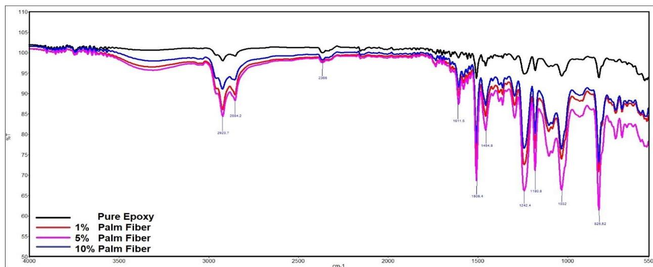
**Figure 3** FTIR graphs of pure epoxy, 1%, 5%, 10% Palm fiber reinforced epoxy composites
