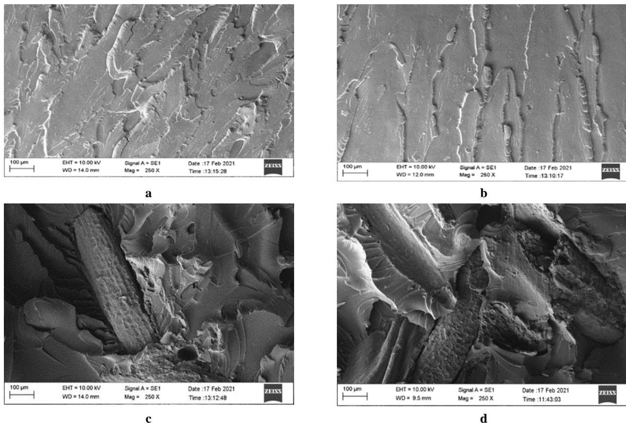
**Figure 4** SEM micrographs of a-) Pure epoxy, b-)1%, c-)5%, d-)10% Palm fiber reinforced epoxy composites
