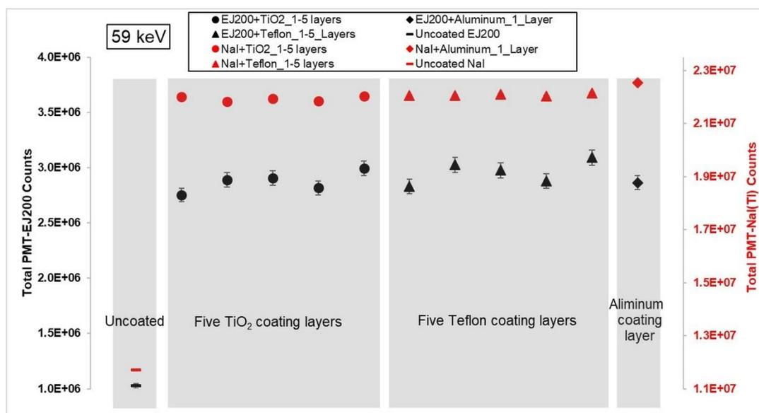
**Figure 3.** 59 keV gamma photons directed to the scintillator from 5 cm away from middle-top of it. PMT counts were recorded for 20000 gamma events and the standard deviations were calculated.
