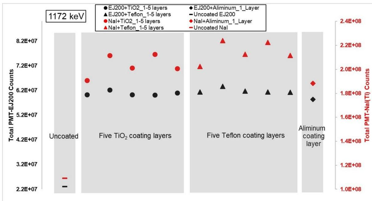
**Figure 5.** 1172 keV gamma photons directed to the scintillator from 5 cm away from middle-top of it. PMT counts were recorded for 20000 gamma events and the standard deviations were calculated.
