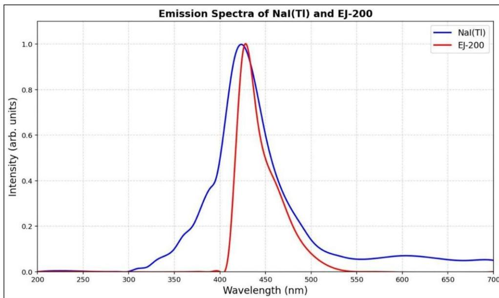
**Figure 1.** Emission spectra of two different scintillators used in this study.
