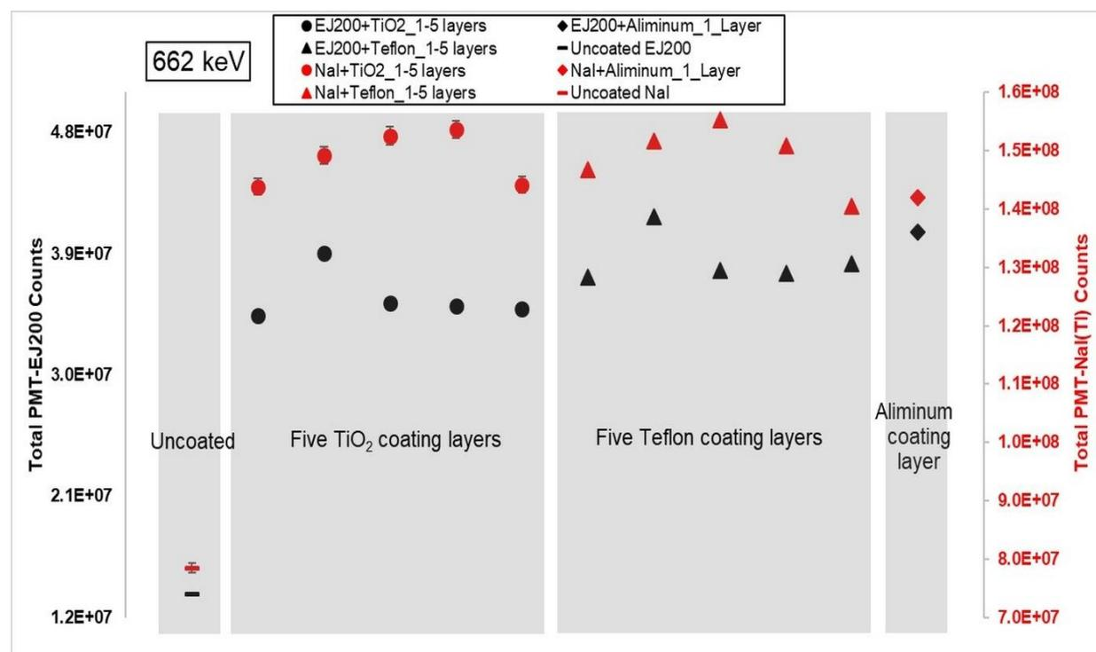
**Figure 4.** 661 keV gamma photons directed to the scintillator from 5 cm away from middle-top of it. PMT counts were recorded for 20000 gamma events and the standard deviations were calculated.
