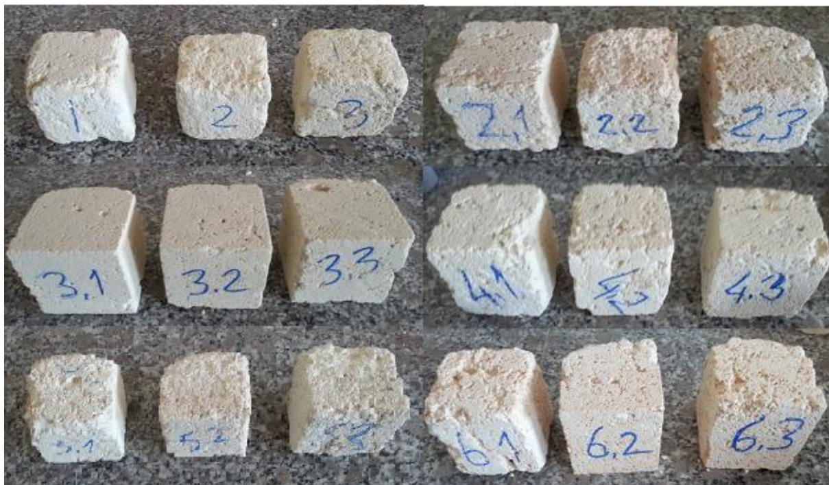
Figure 5. Degraded specimens after salt crystallization experiments
