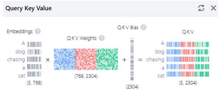
Figure 11. Demonstration of QKV Calculation for the Given Prompt
