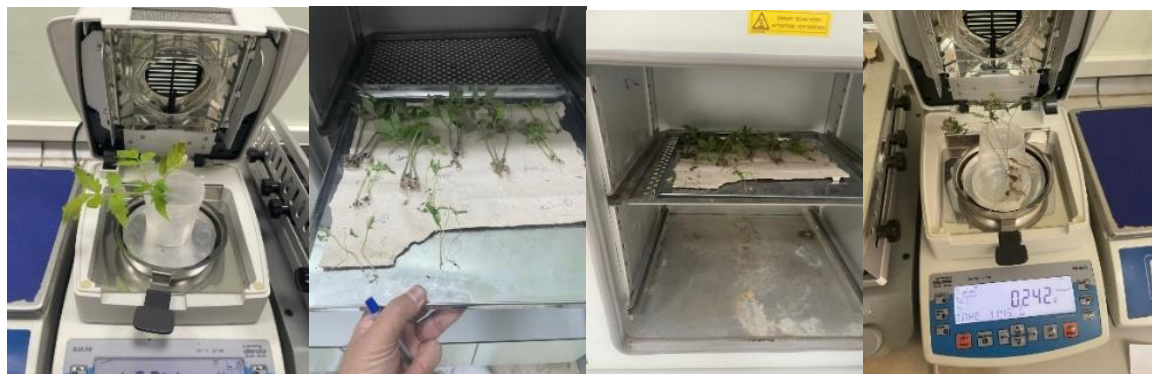
Figure 4. Weight measurement and drying processes for moisture determination of plants.
