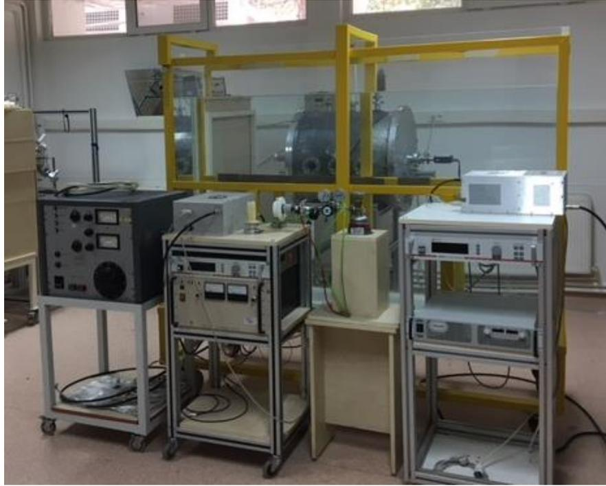
Figure 1. A view of the cylindrical IEC device with all components
