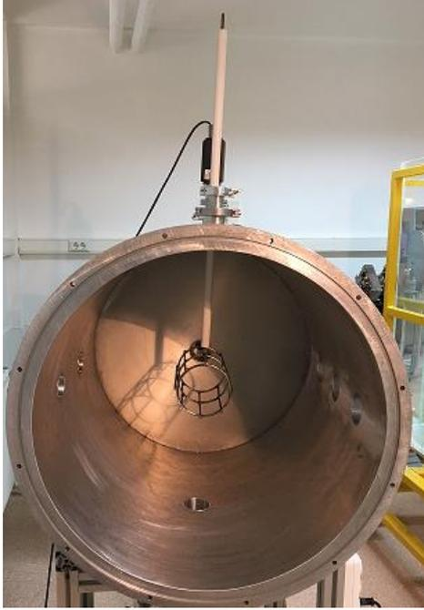
Figure 1a. The cathode with insulator and anode
