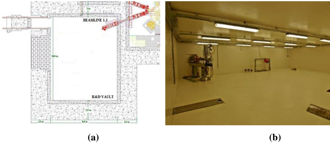
Figure 1. TAEA-PAF R & D irradiation vault and Beamline 1.1 just after construction; (a) The layout plan (b) The photo of the regarding general view.
