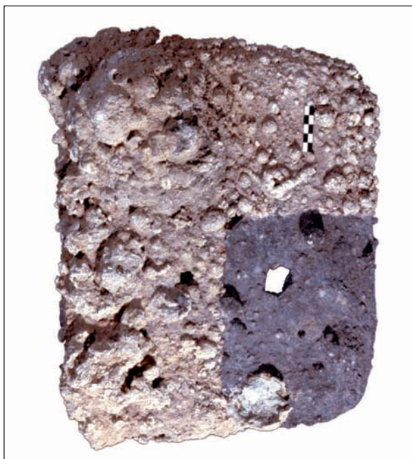
Fig. 4. Rectangular slab ingot (KW 2915) with corner cleaned of marine encrustation, revealing original surface of ingot blemished with corrosion "warts". Note chisel-punched hole at center of cleaned section.
