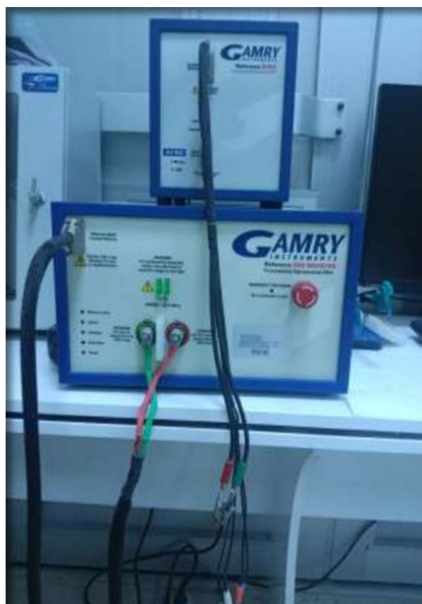
Figure 1. GAMRY Reference 3000 potentiostat device
